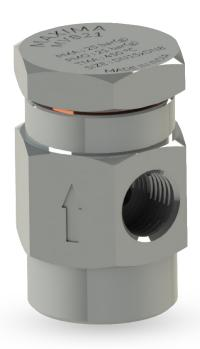
Maxima's MVB21 Vacuum Breaker Series is specifically designed to safeguard heat exchangers, jacketed vessels, kettles, serpentine systems against vacuum created due to condensation of the steam during the process. Due to steam condensation in these systems pressure suddenly decreases and in extreme conditions vacuums are created. The vacuum breaker breaks the vacuum by pushing air into the system.
